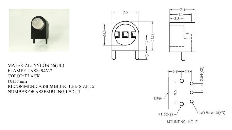
To weld  $\varphi 5$  3PIN LED on board 90 degrees, with same height, and indexing pins, but avoid crooked.
