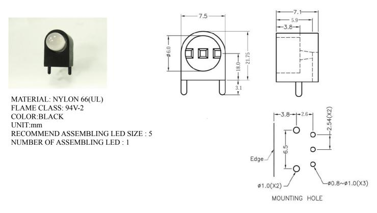
To weld  $\varphi$ 5 3PIN LED on board 90 degrees, with same height, and indexing pins, but avoid crooked.
