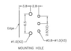
To weld  $\varphi 5$  3PIN LED on board 90 degrees, with same height, and indexing pins, but avoid crooked.
