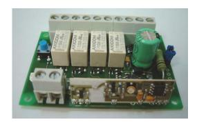
The decoder board HCS-DEC-4 is a 4 channels central unit which can be matched with any HCS Keeloq encoded keyfob programmed with Aurel manufacturer code.
