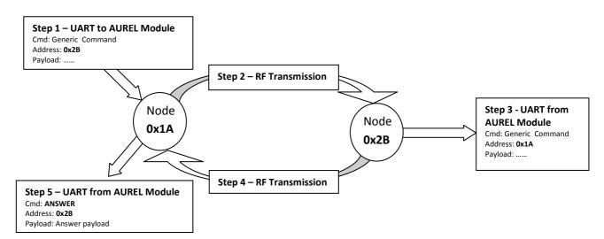
A communication is started through the issue of a generic command through the UART from the external microcontroller to Aurel module. The packet is delivered through the network to the destination node and it is redirected to UART. Successively a answer packet (Command: **ANSWER**, with a specific answer payload) returns to the first node and it is also redirected to UART.
