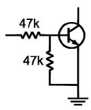
In order to reduce power consumption when the module is switched off take care of the input/output state at power-down, thus avoiding undesired current flow on the bias resistors. Similarly to +3V if a button is to be used add a pull-up (or pull-down) resistor properly.
