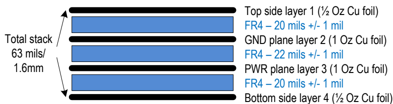
Figure 2-2 SP140 board stack-up
