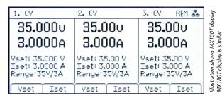
The illuminated keypad includes six soft keys via which voltage or current can be instantly set for any output, or which can be used to set up other functions using a menu system.
