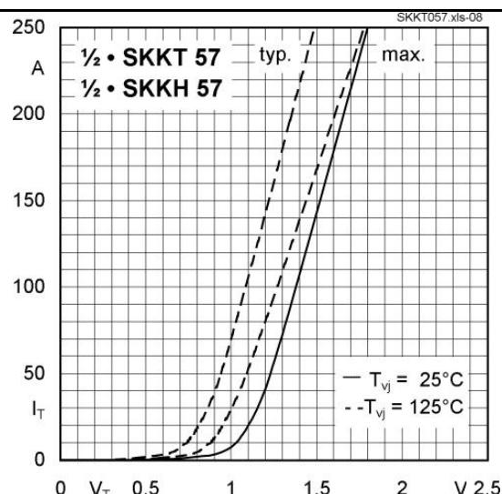
Fig. 7 On-state characteristics
