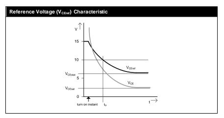
After  $t_{b1}$  has passed, the V<sub>CE</sub> monitoring will be triggered as soon as  $V_{CE} > V_{CEref}$  and will turn off the IGBT. The error memory will be set, and the output PRIM\_nERROR\_OUT changes to the HIGH state. Possible failure modes are shows in the following pictures.
