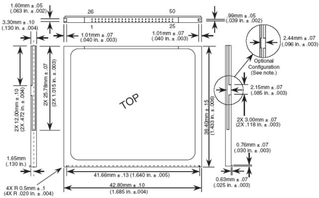
Note: The optional notched configuration was shown in the CF Specification Rev. 1.0. In specification Rev. 1.2, the notch was removed for ease of tooling. This optional configuration can be used but it is not recommended.
