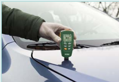
Measuring the thickness of automotive paint
