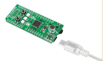
Once you connect the SpeakUp to your computer you're just a few clicks away from configuring it. The set-up process is dead simple. Launch the application, and it will lead you through the initial steps of recording and assigning commands.
