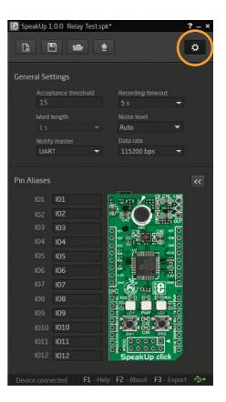
Noise level: Minimal sound volume level that can trigger a voice command recognition. Lower values require quieter pronunciation, resulting in higher noise/hiss sensitivity. On the contrary, higher level values require louder pronounciation and they are less sensitive to noise/hiss.
