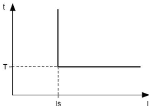
Figure 1.4 - Principle of protection with an independent time delay
