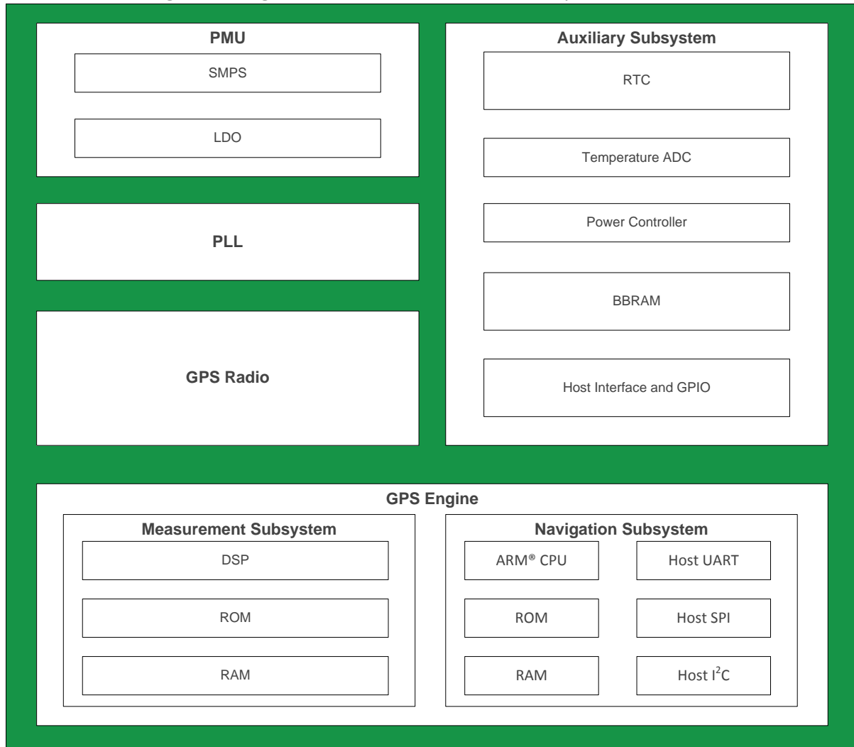
FIGURE 2 – SiRFstarIV™ GSD4e GPS SoC BLOCK DIAGRAM
