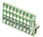
This module enables visual checking of the states on microcontroller leads or integrated circuit leads. In addition, in a simple and visual way you can check bit operations, such as logical shifts (left and right shifts), sum, product and so on.
