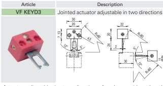
Actuator adjustable in two directions for doors with reduced dimensions.
