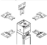
Removing the two fastening screws, in all switches, the head can be rotated in 90° steps.
