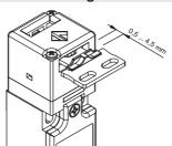
This switch has a wide backlash of the actuator into the head (4 mm) for an easier installation. With closed door, check that the actuator doesn't knock straight against the head of the switch; it must be in the adjustment zone
