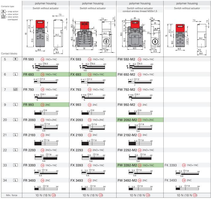
All switches listed above are available in the version with 30N actuator extraction force. To obtain these products, the order code has to be changed adding the extension "-E3", for example FR 693-E3.
