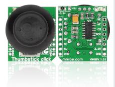
Thumbstick click<sup>™</sup> is a simple solution for adding an analog thumb joystick to your design. Along with the dual axis joystick unit, the board also carries an **MCP3204** 12-bit A/D converter. Thumbstick click<sup>™</sup> communicates with the target board microcontroller through **mikroBUS<sup>™</sup>** SPI (CS, SCK, MISO and MOSI) lines. The board is designed to use either a 3.3V or a 5V power supply.
