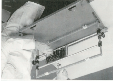
Unslotting of components carried out with PC Assembly Jig in vertical positions.
