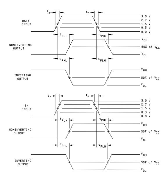
FIGURE 4. Switching waveforms and test circuit.
