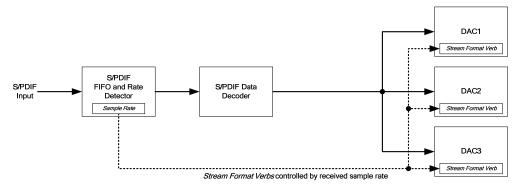
Figure 17 S/PDIF Receive to DACs
