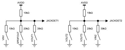
Figure 24 Required Jack Detect Components
