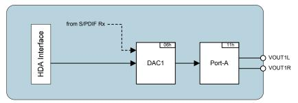
Figure 11 Stereo Headphone Playback Path
