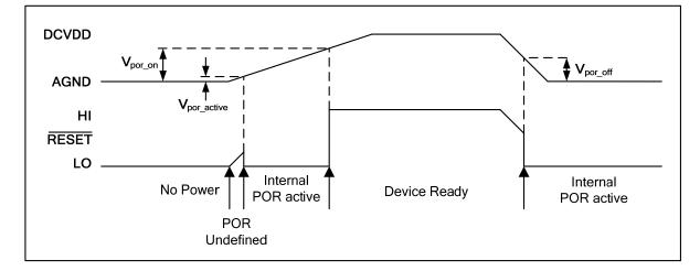
Figure 3 Typical Power up Sequence
