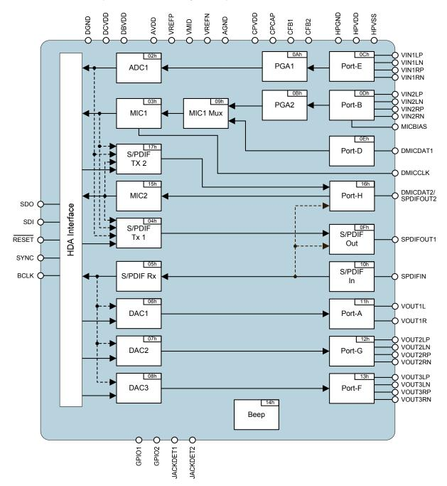
Figure 4 Widget Diagram Showing Valid Audio Paths
