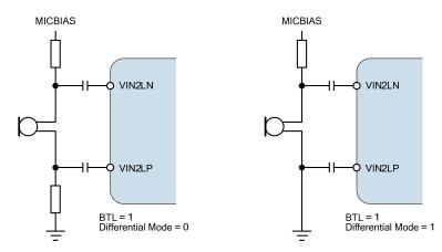
Figure 8 Port-B Example External Connections (one channel shown)
