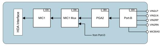
Figure 7 Stereo Analogue Microphone Record Path
