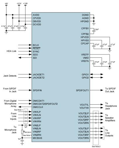
Figure 23 Recommended External Components
