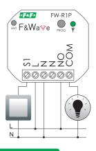
S1 - control input triggered with level L or N
