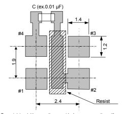
To maintain stable operation, provide by-pass capacitor with more than 0.1  $\mu\text{F}$  at a location as near as possible to the power source terminal of the crystal products (between VCC - GND).
