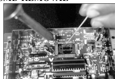
2. With a soldering iron, melt ChipQuik low temperature alloy
