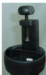
Clamp Fitted to Base
