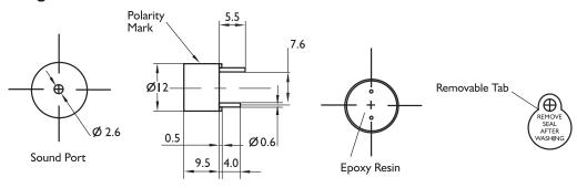
Dimensions : Millimetres Tolerance : ±0.5mm
