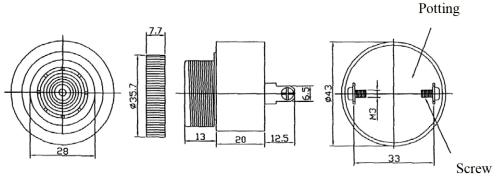
Dimensions: Millimetres Tolerance: ±0.5mm
