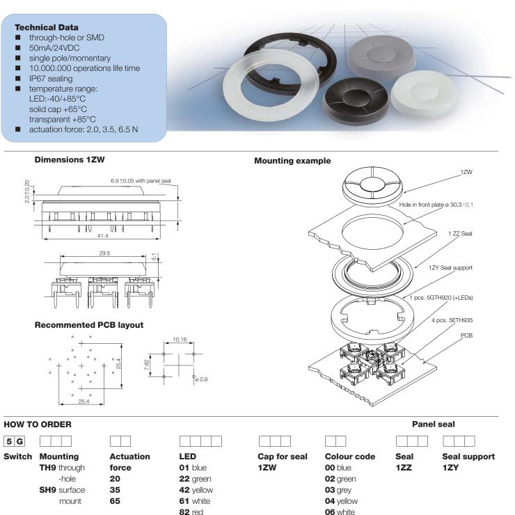
Dimensions (mm) Unless otherwise specified, all tolerances ±0,2 Ordering example (sealed version) 1ZW: 1 x 5GTH920 + 4 x 5ETH935 + 1ZW03 + 1ZZ + 1ZY
