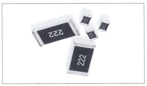
made by electroplating. plating is fired on and the strips broken into individual components. Final termination is resistor is trimmed to tolerance by laser. The pre-scribed tile is broken into strips, the end resistive element is screen printed and fired and the passivation layer added. Each Precious metal terminations are screen printed onto a ceramic base and fired. The
