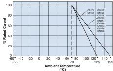
For resistors operated at an ambient temperature of 70°C or above, a power rating shall be derated in accordance with the above derating curve.
