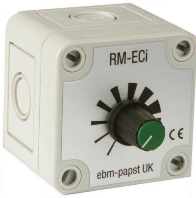
The RM-ECi controller is for use with the full range of ebm-papst EC fans. Powered by the 10VDC output from the motor, it provides infinitely variable, manual speed control between 0% and 100%.
