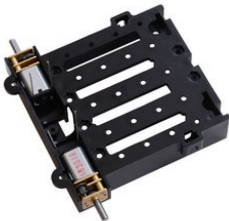
Zumo chassis being assembled with two micro metal gearmotors.
