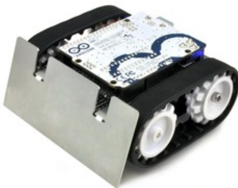
Assembled Zumo robot with a Zumo Shield, Arduino Uno, and Zumo blade.
