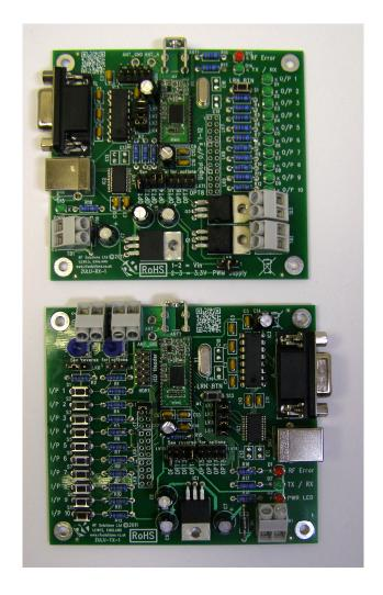
The Evaluation boards are sold as a TX and RX PCB pair, ready for component population. Schematics are shown below, not all components are fitted for each of the projects.
