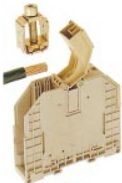
Open terminal cover, remove screw terminal unit
