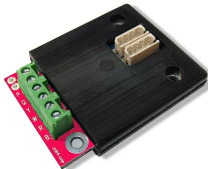
The A2P interface is a 0-10 volt to open collector PWM converter and is designed to work with ebm-papst 4 wire PWM controlled DC fans. The interface translates the analogue voltage input to an equivalent PWM signal. The interface is matched to the fan so that with its very low power consumption, there is no need for a separate dedicated power supply.
