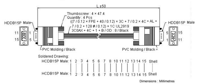
Cable Word : E210567 AWM 2919 80°C 30 V VW-1 ......C AWM A I/II 80°C 30 V FT1 Low Voltage Computer Cable Kaibo
