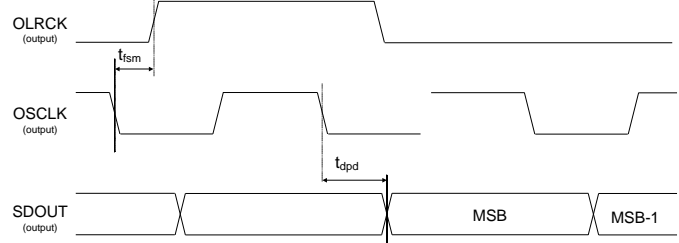
Figure 4. TDM Master Mode Timing
