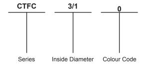
Inside Diameter : Expanded as supplied/Recovered after heating.
