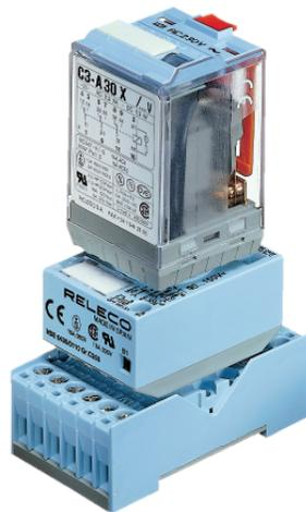
The modules **CT 2** and **CT 3** are electronic timers that are designed to be inserted between a standard plug-in relay and its socket, enabling the relay to be operated as a timer relay.
