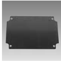
Mounting plates Laminated paper (Pertinax) (thickness: CT-50 to CT-60: 1.5 mm; CT-62 to CT-78: 2.0 mm; CT-80 to CT-91: 2.5 mm), can be used for subsequent mounting of equipment.
