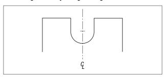
For heatsink lengths from 88mm to 150mm three notches in each flange 38mm apart.
