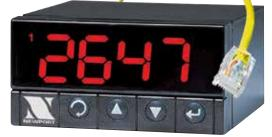
current ranges. The iS has built-in 5 or 10 Vdc excitation for bridge transducers, 5 Vdc @ 40 mA or 10 Vdc @ 60 mA (any excitation voltage between 5 and 24 Vdc is available by special order). This iS model supports 4- and 6-wire bridge configurations, ratiometric and non-ratiometric measurements.
