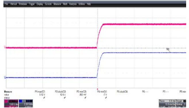
Figure 37 – Output Voltage and Current Waveforms. 265 VAC Input. Upper: 5 V, 2 V / div. Middle: I_{OUT} , 1 A / div. Lower: 12 V, 5 V, 1.6 ms / div.
