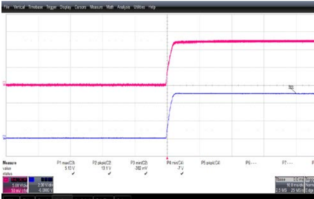
Figure 38 – Output Voltage and Current Waveforms. 85 VAC Input. Upper: 5 V, 2 V / div. Middle: I_{OUT} , 1 A / div. Lower: 12 V, 5 V, 1.6 ms / div.
