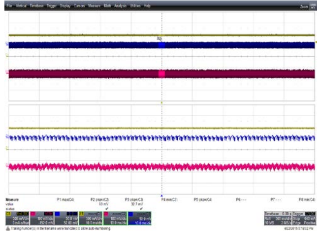
Figure 49 – Output Ripple Voltage Waveforms. 265 VAC Input. 1.0 A on 12 V. 5 V PK : 33 mV, 12 V PK : 93 mV. Upper: 5 V, 50 mV / div. Lower: 12 V, 100 mV /, 500 ms, 20 ms / div.
