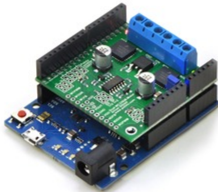
Pololu dual MC33926 motor driver shield, assembled and connected to an Arduino Leonardo.
