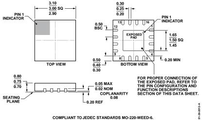
Figure 10. 16-Lead Lead Frame Chip Scale Package [LFCSP\_WQ] 3 mm × 3 mm Body, Very Very Thin Quad (CP-16-27) Dimensions shown in millimeters
