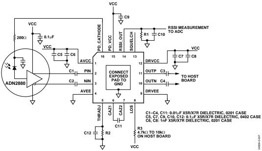
Figure 8. Typical ADN2890 Applications Circuit
