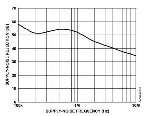
Figure 5. Typical PSRR vs. Supply-Noise Frequency
