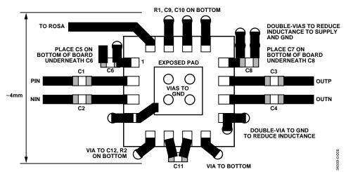
Figure 9. Recommended ADN2890 PCB Layout
