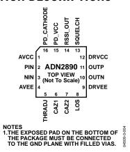
Figure 2. Pin Configuration
