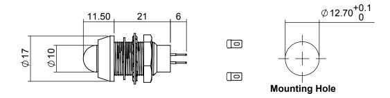
Anode termination indicated by red sleeve. Mounting hole to be clean and burr free.
