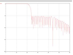
Figure 61 DAC Filter Response (fs=32kHz)
