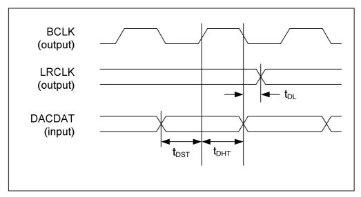
Figure 2 Digital Audio Data Timing - Master Mode
