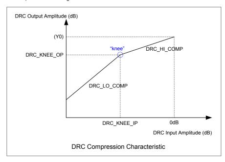
Figure 25 DRC Compression Characteristic
