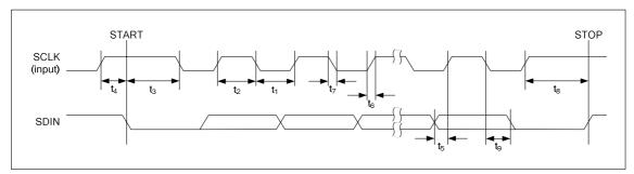
Figure 4 Control Interface Timing – 2-Wire Serial Control Mode
