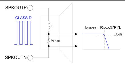
Figure 68 Speaker Equivalent Circuit
