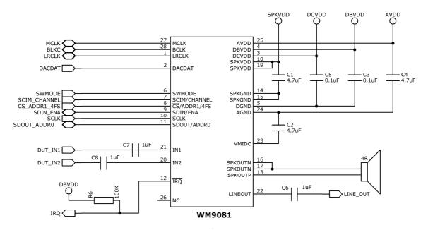
Figure 67 Recommended external components
