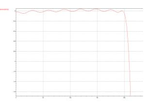
Figure 65 DAC Filter Response (fs=96kHz)
