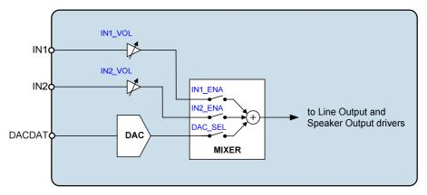
Figure 32 Input Signal Mixing
