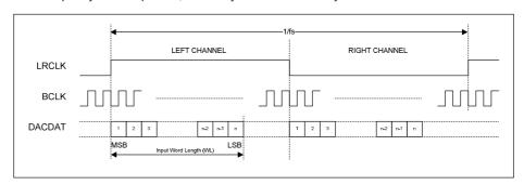
Figure 40 Left Justified Audio Interface (assuming n-bit word length)
