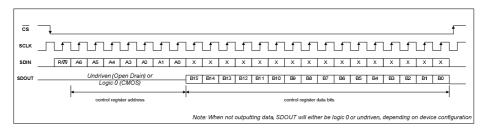
Figure 19 4-Wire Serial Control Interface
