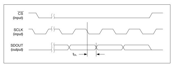
Figure 8 Control Interface Timing – 4-Wire Serial Control Mode (Read Cycle)
