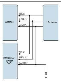
Figure 38 TDM with Processor as Master
