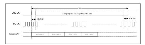
Figure 50 TDM in DSP Mode B - 2 Stereo Time Slots
