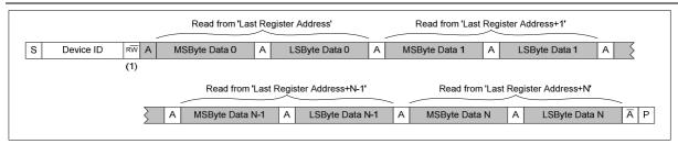
Figure 17 Multiple Register Read from Last Address using Auto-increment
