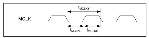
Figure 1 System Clock Timing Requirements
