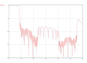
Figure 57 DAC Filter Response (fs=12kHz)
