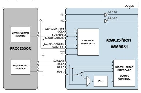
Figure 10 Software Control Mode Example – 2-Wire Control, Slave Mode, Device ID = D8h
