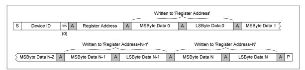
Figure 15 Multiple Register Write to Specified Address using Auto-increment
