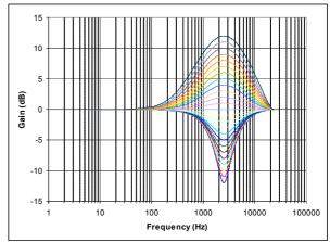
Figure 28 EQ Band 3 - Peak Filter Response
