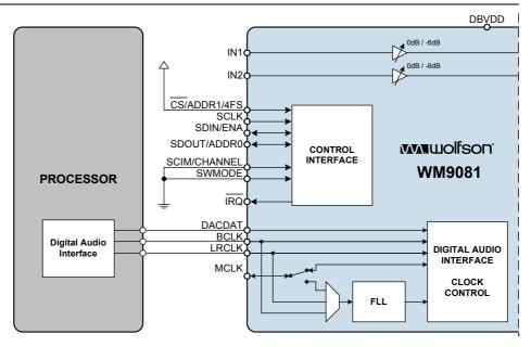
Figure 21 Hardware Control Mode Example - 4FS Mode, Left Channel
