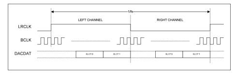
Figure 46 TDM in Right-Justified Mode - 2 Stereo Time Slots
