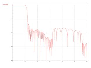
Figure 58 DAC Filter Response (fs=16kHz)
