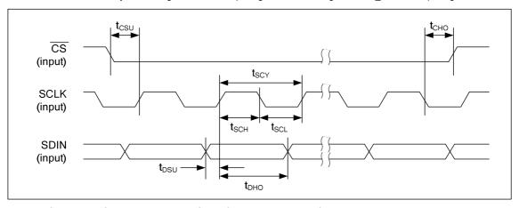
Figure 5 Control Interface Timing – 3-Wire Serial Control Mode (Write Cycle)
