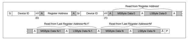
Figure 16 Multiple Register Read from Specified Address using Auto-increment
