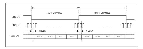
Figure 48 TDM in I<sup>2</sup>S Mode - 4 Stereo Time Slots
