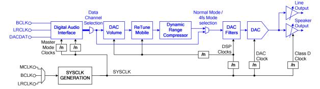
Figure 9 DAC Signal Path and Clocking Architecture
