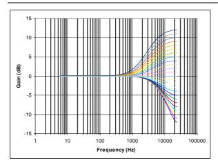
Figure 30 EQ Band 5 - High Freq Shelf Filter Response
