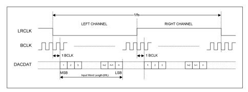
Figure 41 I2S Justified Audio Interface (assuming n-bit word length)
