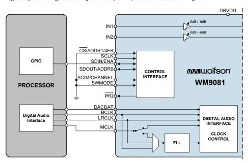
Figure 20 Hardware Control Mode Example - Normal Mode, Left Channel
