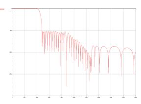
Figure 63 DAC Filter Response (fs=48kHz)
