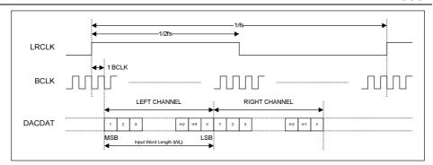
Figure 42 DSP Mode Audio Interface (mode A, AIF\_LRCLK\_INV=0, Master)
