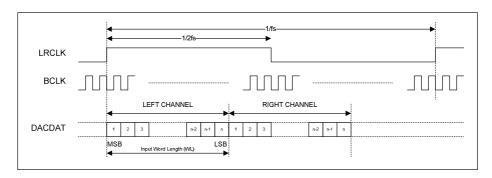
Figure 43 DSP Mode Audio Interface (mode B, AIF\_LRCLK\_INV=1, Master)
