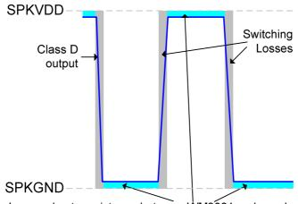
Losses due to resistance between WM9081 and speaker (e.g. inductor ESR) This resistance must be minimised in order to maximise efficiency.
