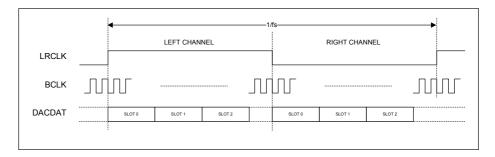
Figure 47 TDM in Left-Justified Mode - 3 Stereo Time Slots
