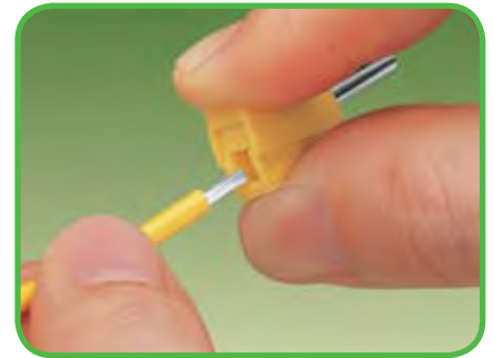
Connection of conductors: Press button fully and insert stripped conductor into square entry and release
