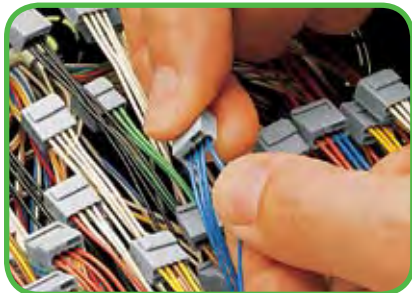
Removal: Hold wire to be removed and twist alternately left and right while pulling the connector
