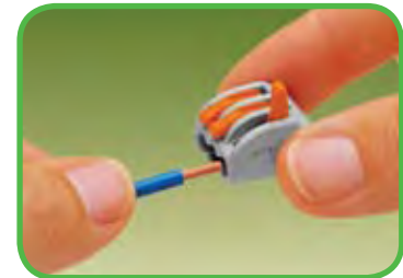
3) Insert conductor and push down lever
