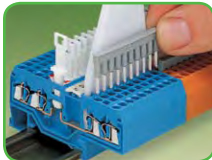
Commoning of front-entry through terminal blocks with comb type jumper bars with the aid of a 10-way operating tool
