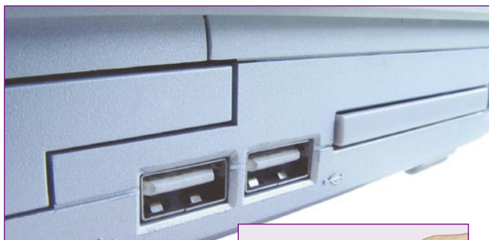
USB type A connector - at a PC/notebook or hub
