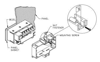
While holding the unit in place, push the panel latch over the rear of the unit so that the tabs of the panel latch engage in the slots on the case. The panel latch should be engaged in the farthest forward slot possible. To achieve a proper seal, tighten the latch screws evenly until the unit is snug in the panel (Torque to approx. 28 to 36 in-oz [0.202 to 0.26 N-m]). Do not over-tighten the screws.
