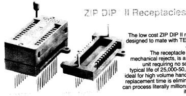
The low cost ZIP DIP II receptacle series is designed to mate with TEXTOOL's series of ZIP DIP II sockets.
