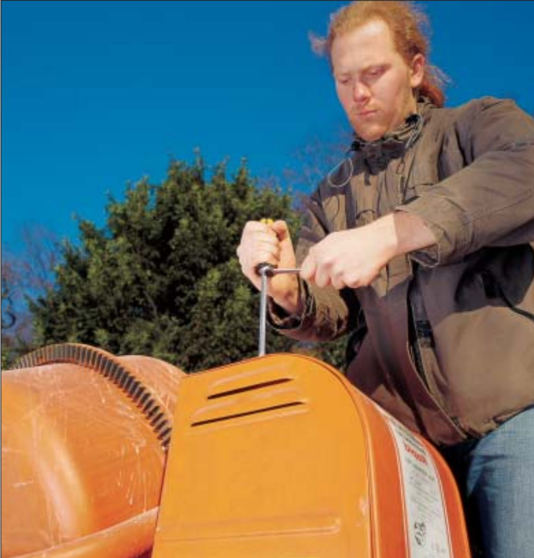
The hex bolster allows for the use of an open-jawed or ring spanner, to transfer higher torque.
