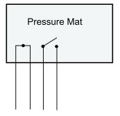
In a 4 wire configuration the two wires on the far left are the tamper loop. These are only needed when connecting to an alarm control panel.
